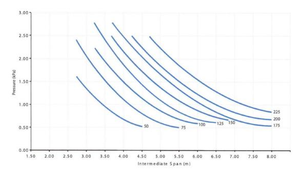
Note: Allowable wind pressure is in accordance with AS1170.2 for permissible stress analysis Factor of Safety is 1.80 on ultimate.
